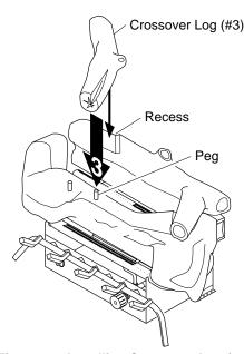
Figure 23 - Installing Crossover Log (#3)
